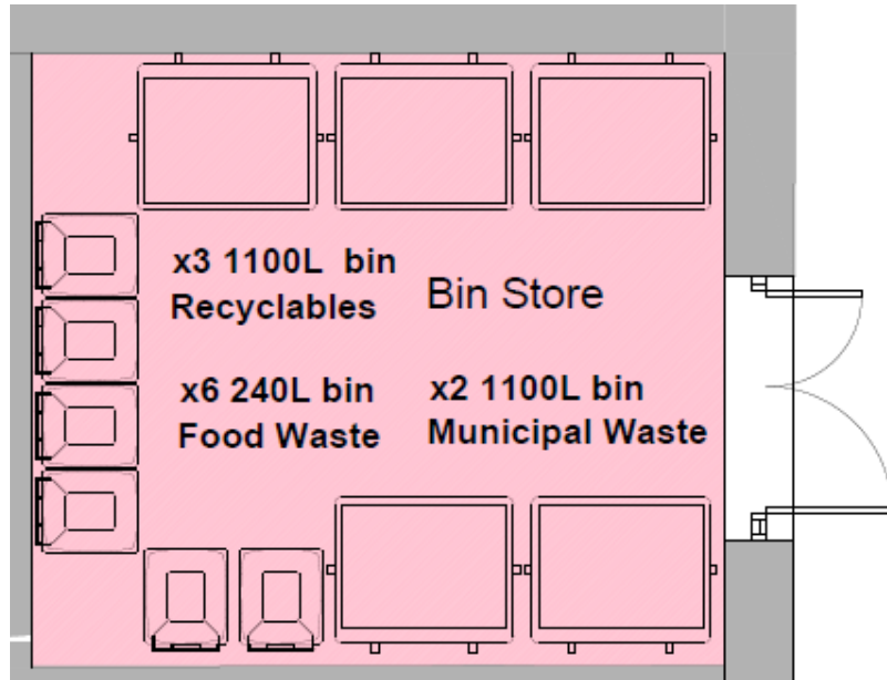
Figure 4-3 Bin Stores in Block C
